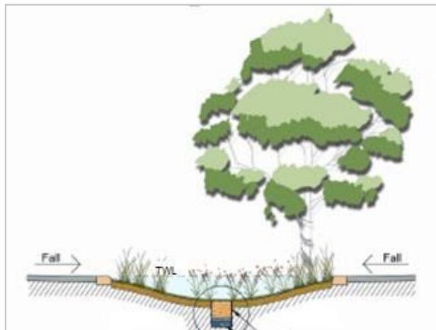
Figure 3.6: Indicative vegetated swale cross section
