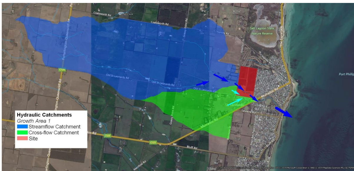
Figure 1.4: Ibbotson Street site (Growth Area 1) – hydraulic catchments
